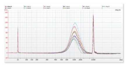
**Figure 4:** Bioanalyzer traces from the libraries prepared on Biomek NGeniuS system 10 ng run.
