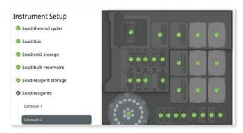
**Figure 3b. Deck setup:** A step-by-step series of prompts is directed by the application with the Dynamic DeckOptix system confirming correct labware placement while advancing steps through to completion in real-time.
